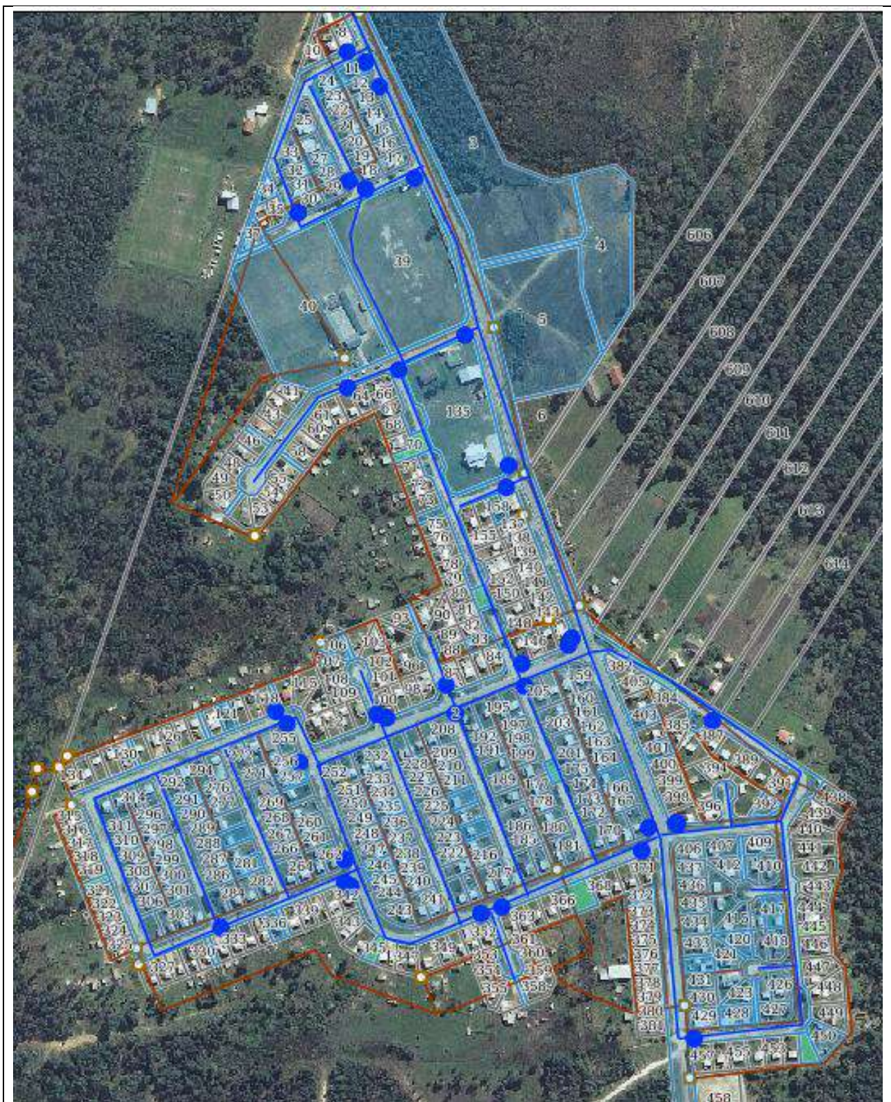
Figure 3: Existing Sewer Reticulation, Woodlands Settlement (SMEC, July 2025)
